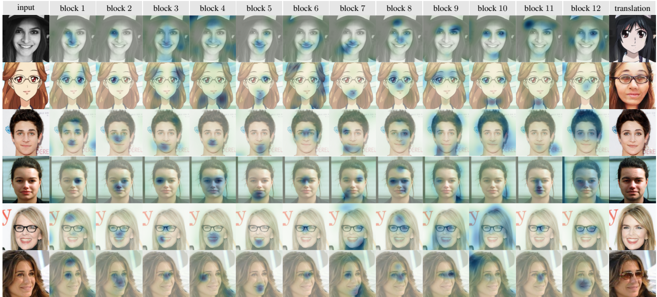
Figure 4. Attention. Attention heatmap generated by the attention weights from the 12 Transformer encoder blocks in the pixel-wise ViT. The attention heatmap demonstrates the amount of attention different locations of an image receive.
